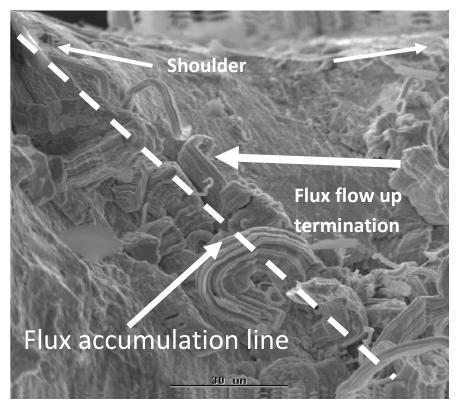
Figure 3 - SEM Image of SOT gull wing termination
