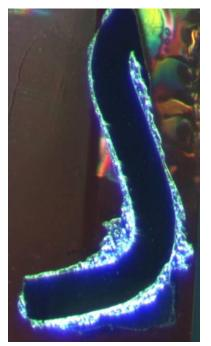
Figure 8 – Optical Image of primary whisker in cross-section
