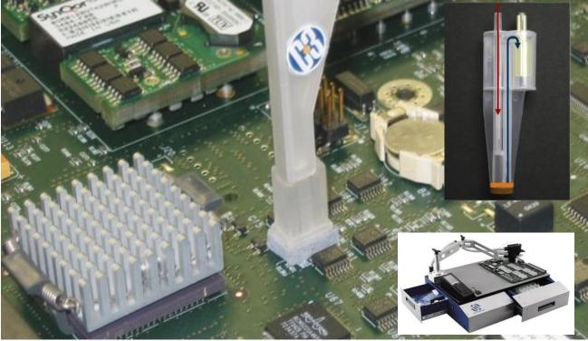
Figure 11 – Cleanliness test system
