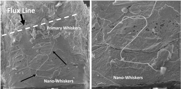
Figure 4 & 5 - SEM Image of primary and Nano-Whiskers
