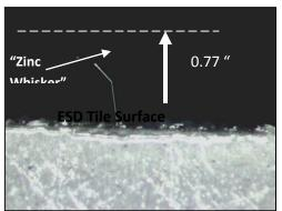
Figure 1 - Tin whisker on zinc alloy ESD floor time
