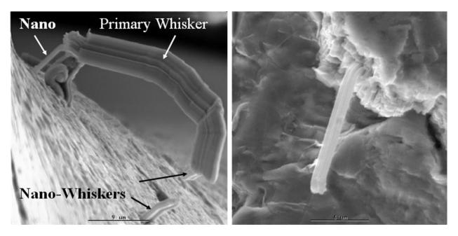
Figure 6 & 7 - SEM Image of primary and Nano-Whiskers
