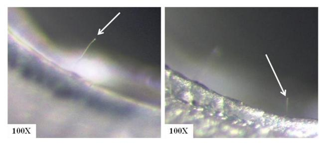
Figure 18 & 19 – optical images of whiskers on jack screw threads
