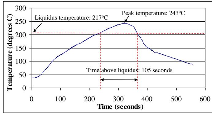
Figure 2: Lead-free reflow profile used for the exposures
