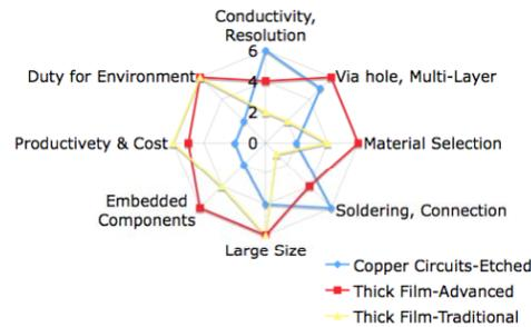
Fig. 1 Comparison of the circuit manufacturing processes
